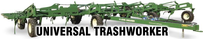
10", 12" & 13.1" SPACINGS - 29', 35' & 41' WORKING WIDTHS
