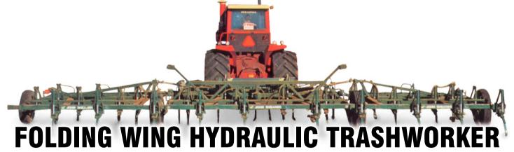
FEATURES - Four (4) row main frame - Edge-on tyne 50mm x 32mm (2" x 1¾") - Robust 100mm x 100mm main frame - Hydraulic tyne loading - Tyne Spacings: 305mm (12") or 254mm (10") - Tyne breakout, up to 454kgs (1,000lbs) - 770mm underframe clearance - Induction hardend pins (35mm) and bushes - Maximum working depth, 360mm
